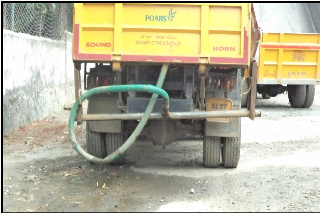
Photographs showing sprinkler system installed in the crusher unit and tipper lorry
