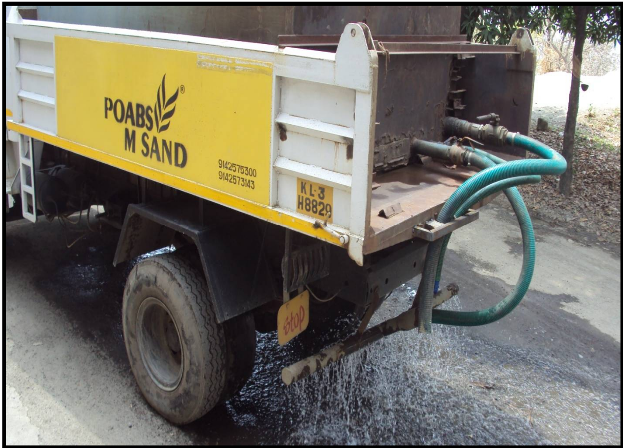
Photograph showing watering on road through sprinkler system installed in tipper lorry
