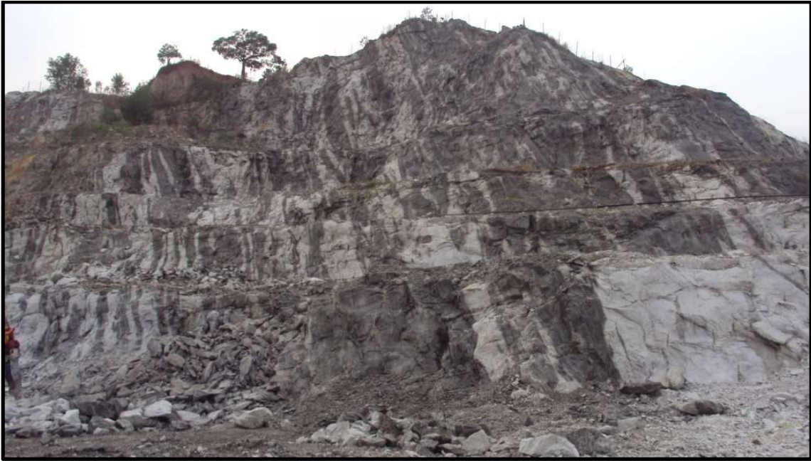
Photograph showing the Bench Type Mining
