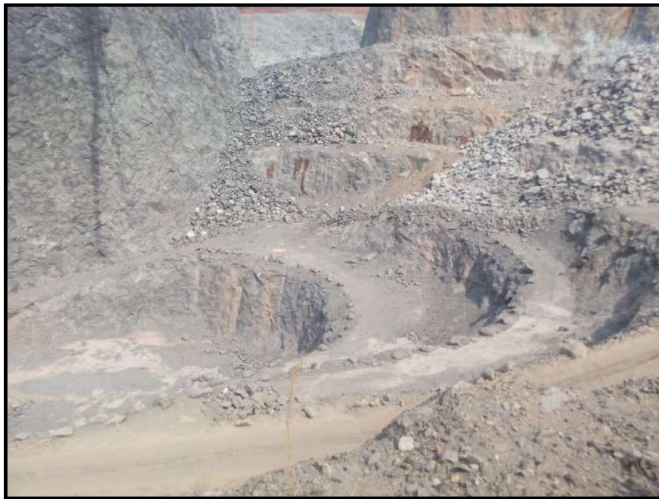
Photographs showing the bench type mining
