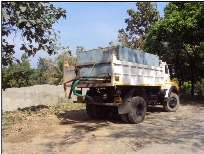
Photograph showing the fixed sprinklers installed in crusher and lorry
