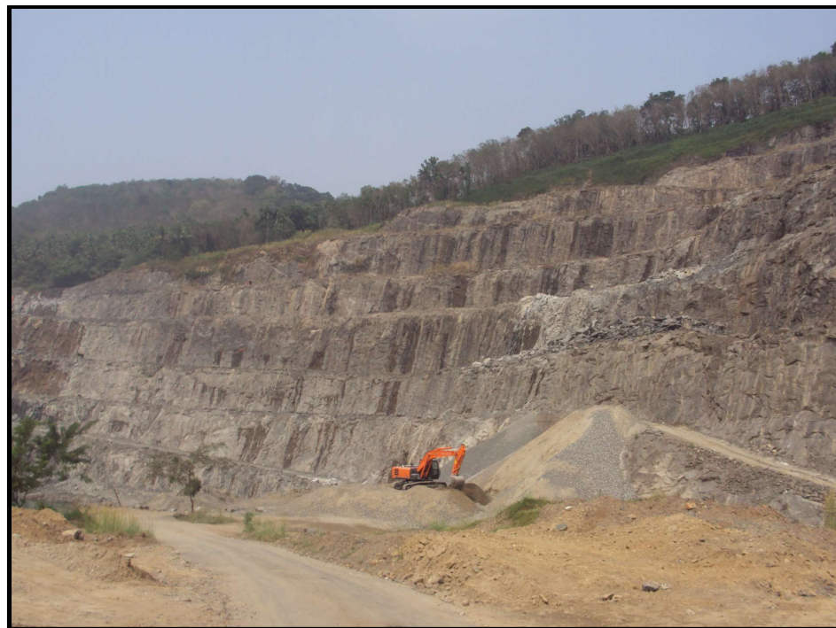
Photograph showing the bench type mode of mining
