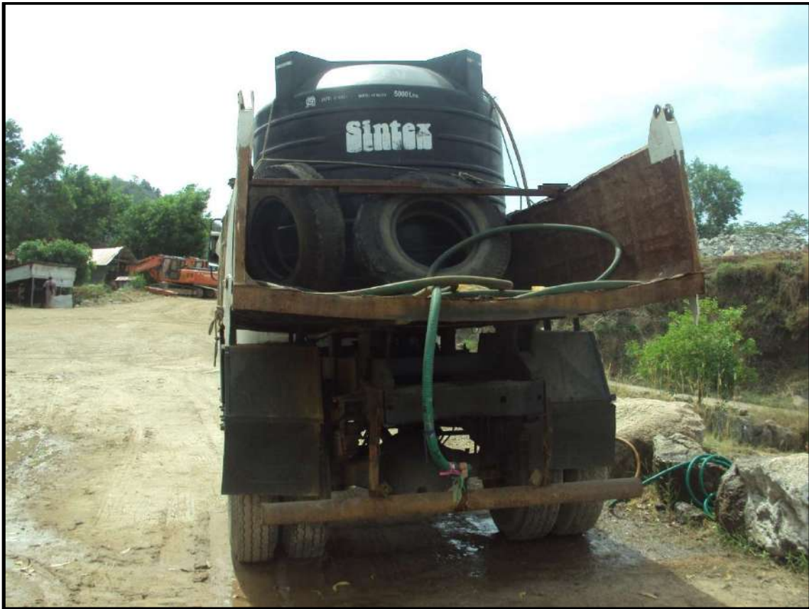
Photograph showing the Sprinkler system installed in tipper lorry
