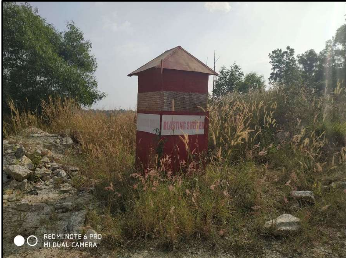
Photograph showing Blasting Shelter installed in the project area
