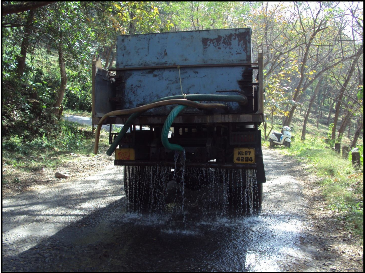
Photograph showing watering on road through sprinkler system installed in tipper lorry
